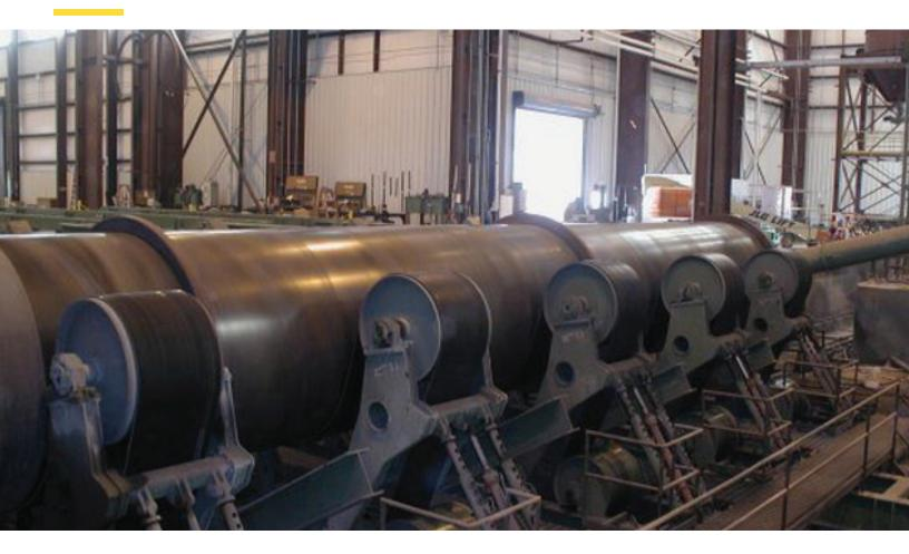
Pipe spinning belts are a truly endless solution for the cement lining process. Built specifically to withstand the weight and high speed spinning of large diameter steel pipe, our truly endless belts will solve any problems with:
